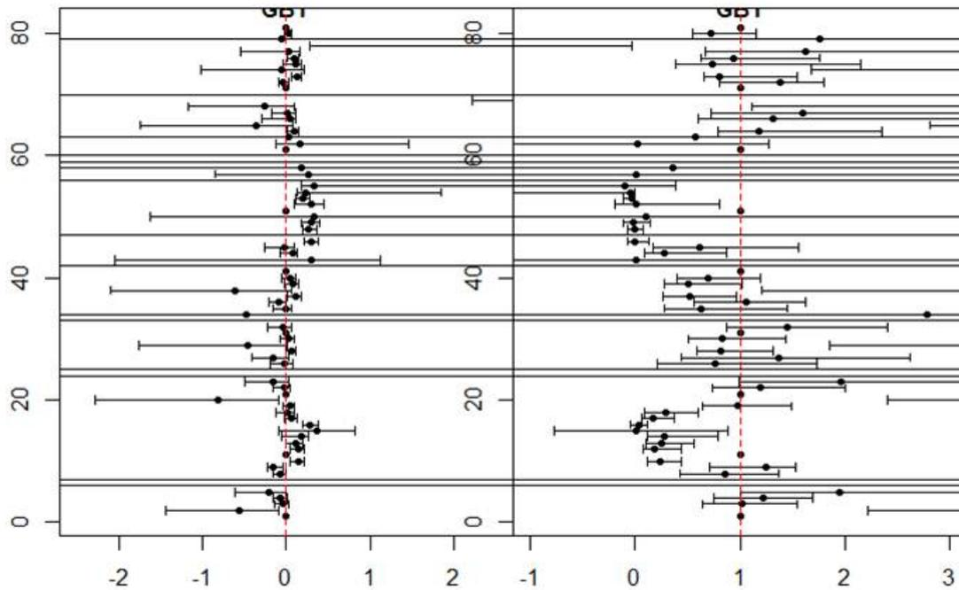
**Figure 6. Centipede plot of the intercept and slope values ( $\pm$ std), of the orthogonal regression plots, for each pod performance comparison in calibration trails at Moneypoint 2011. Deviation from the red dotted lines, 0 on the intercept plot and 1 on the gradient plot, indicates deviation from the null model assuming no variation. Plot indicates that a greater extent of variation is found within the gradient values.**
