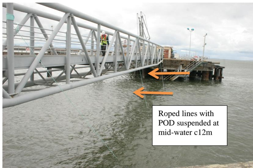
Figure 2. Photograph of mooring used to deploy C-PODs during SAM monitoring in the Shannon Estuary using fixed structures
