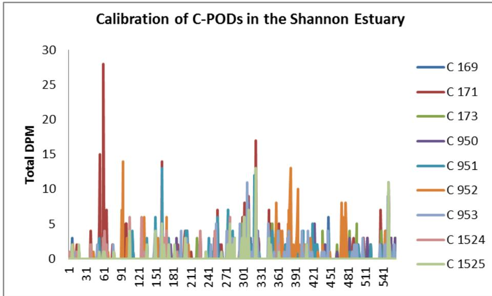
Figure 4. Detection Positive Minutes from units used during the present study, C-PODs 169, 171, 173, 950, 951, 952, 953, 1524, and 1525. C-169 is the reference unit. No correction factor (*cf*) required.
